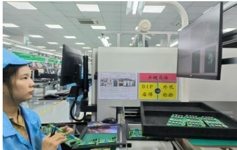
DIP post-furnace AOI 5 sets
