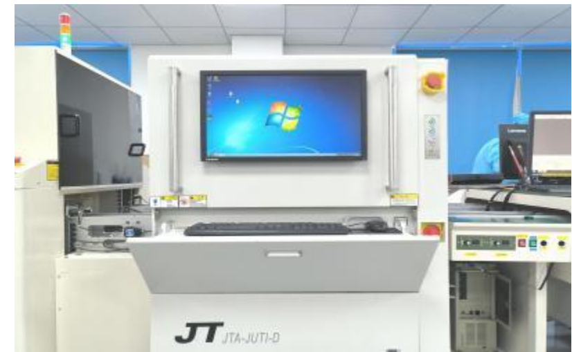
Automatic optical inspection (AOI) 13 sets
